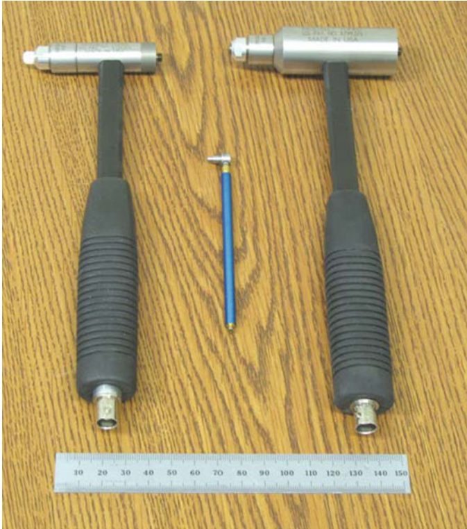
Fig. 7.3 Example impact hammers. A 150 mm steel ruler is included in the photograph to provide scale
